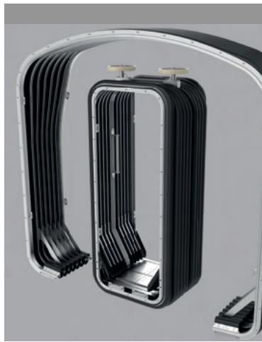
Commuter train gangway with separately latchable inner bellow for maintenance access to jumper cables
