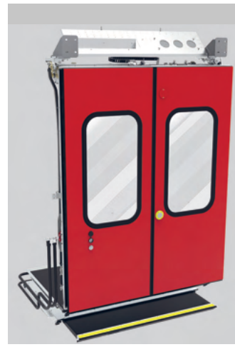
TSI conform plug sliding door with heated sliding steps.
