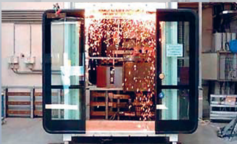
High-voltage test on plug sliding tram door system
